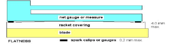
As in thickness measuring, new devices are also available on the market, consisting in a support with a dial in the middle with a pin. The support is placed across the racket in different positions and the pin is placed in the rubber as well. If the rubber is not flat, the dial shall show the difference as it is shown in the figure below.
