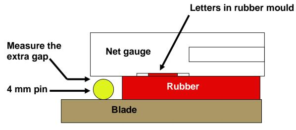
• If the ruler touches the rubber and the pin, but the rubber has a bubble in the middle, the tester has to measure the remaining gap near the pin and at the end of the rubber (see picture below). If the gap near the pin is even or bigger than the gap at the end of the rubber, provided that this gap is less than 0.2 mm, no action shall be taken. If the gap at the end of the rubber is bigger than the gap near the pin and bigger than 0.2 mm, the rubber shall be considered as too thick.
