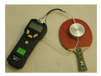
Connect the air outlet tube which is accompanying the instrument to the threaded hole in the right side of the instrument. Then connect the flexible tube to the top part of the instrument. Once both accessories have been connected, each one has to be assembled to the Teflon tubes of the cap.
