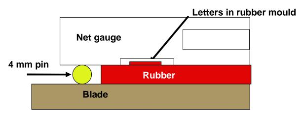
• If the ruler touches the pin and laid-down in the other extreme of the rubber, this is less than 4.0 mm thickness and no action shall be taken.
